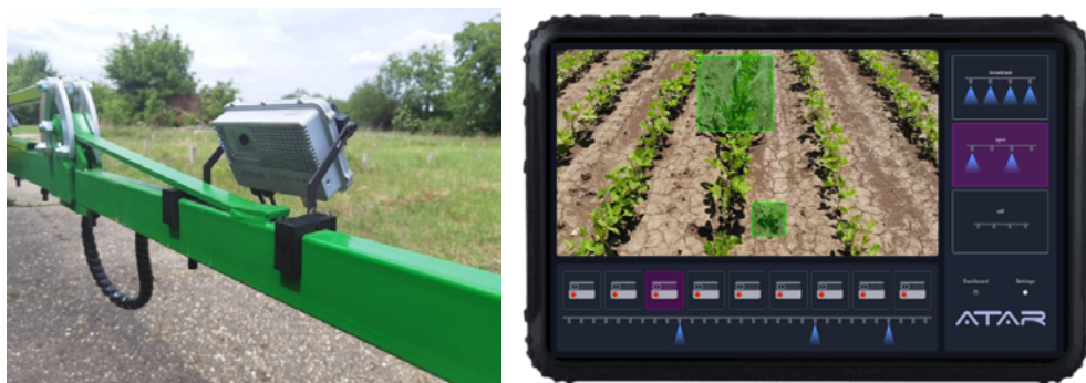
Picture 2. Camera and system that analyze images using a machine learning algorithm to identify weeds in real-time.
