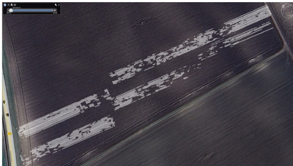
Picture 4. Spraying map in 2024: the area treated with the ATAR smart sprayer system ranged from 29 to 75%.
