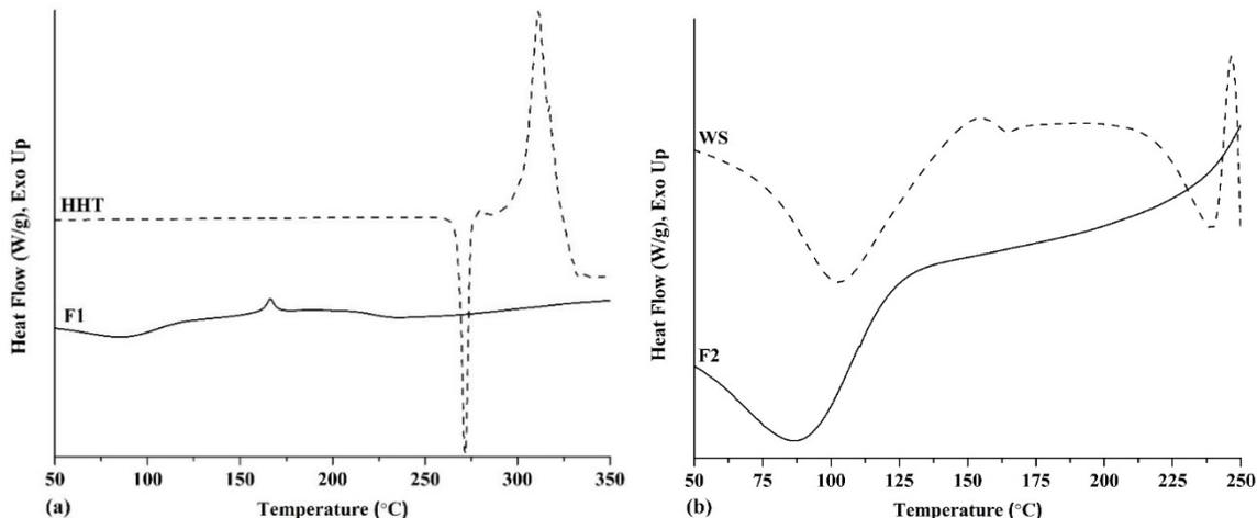
**Figure 3. DSC thermograms of: (a) pure HHT and formulation F1 and (b) pure WS and formulation F2**
