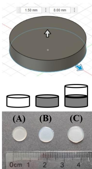
**Figure 1.** Cylindrical 3D model of tablets created in Autodesk fusion software and printed single-layered (A) WS tablets, formulation F2 and (B) HHT tablets, formulation F1 and (C) combined two-layered 3D tablets, formulation CF
