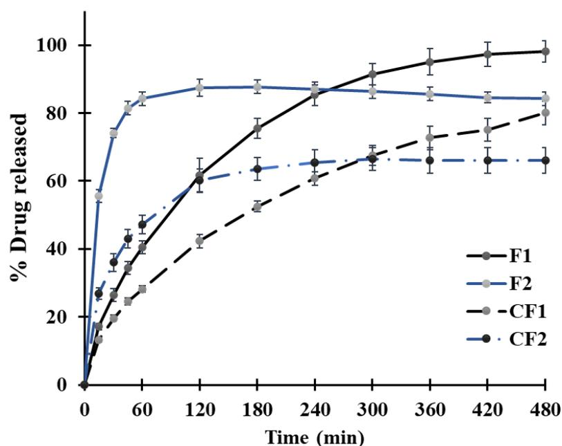
**Figure 2.** Dissolution profiles of fabricated single-layered (F1 and F2) and combined two-layered (CF1 and CF2) 3D tablets
