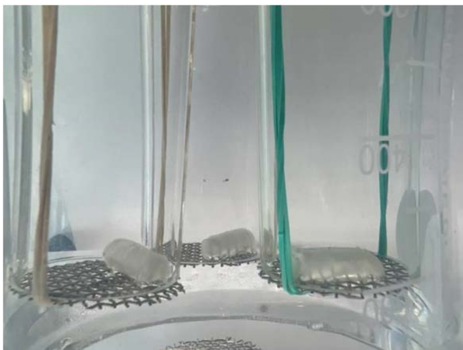
Figure 1. Disintegration method set up to mimic Ph. Eur 2.9.2-1 apparatus
