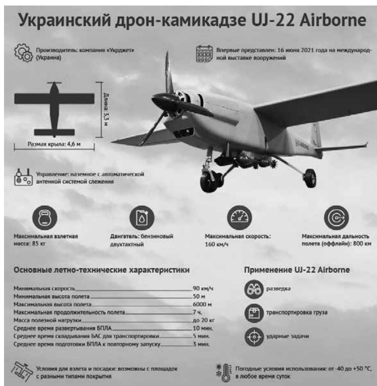
Figure 4: Appearance and characteristics of the UJ-22 attack drone ( https://aif.ru/ , 2023)
