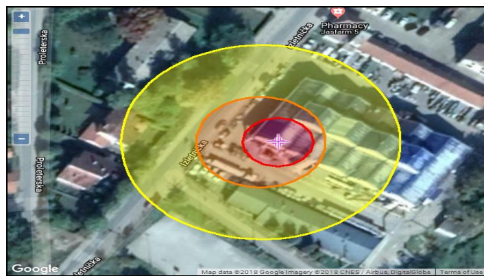
Figure 9. Zones of thermal radiation of acetylene in Scenario 3 in real space.
