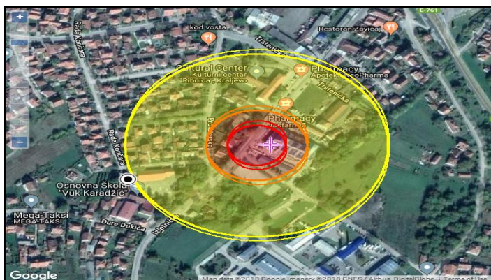
Figure 7. Zones of explosive acetylene cloud spreading in Scenario 2 in real space.
