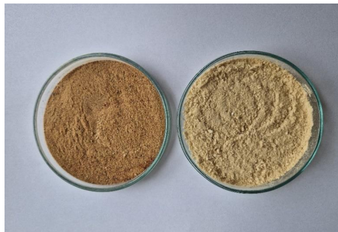
Figure 2. PIs obtained from plum oil cake by thermal (PPIT) and freeze-drying (PPIF)
