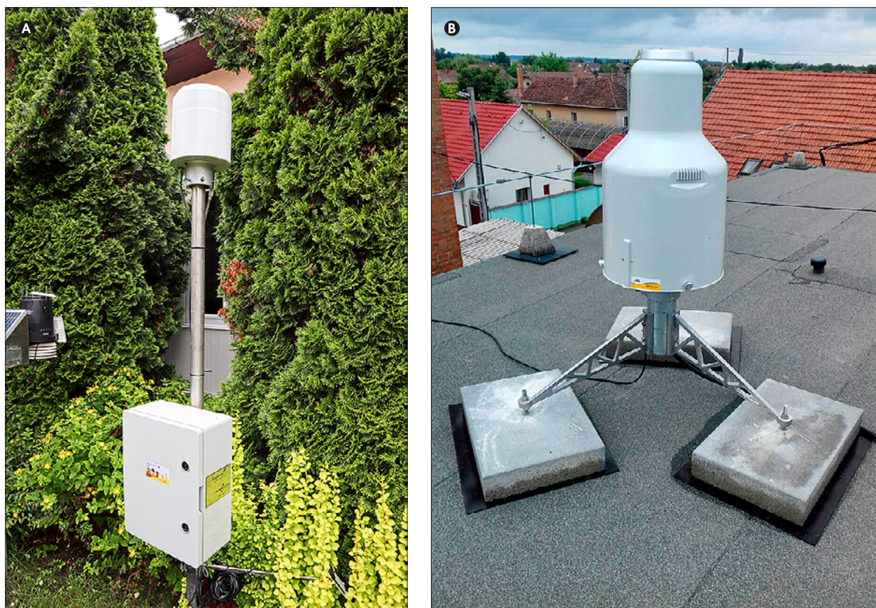
Figure 9. Precipitation sensor types in Novi Sad and Szeged monitoring network, a) Lambrecht rain[e] station in Novi Sad, and b) OTT Pluvio 2 station in Szeged
