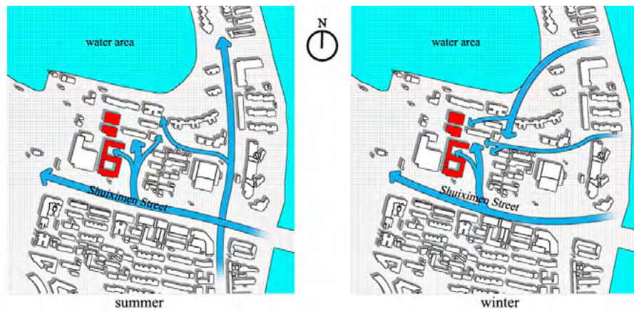
Figure 13. Two scenarios with wind corridors in case of Mochou Lake Primary School are developed in different seasons. School buildings are shown in red (the same below)
