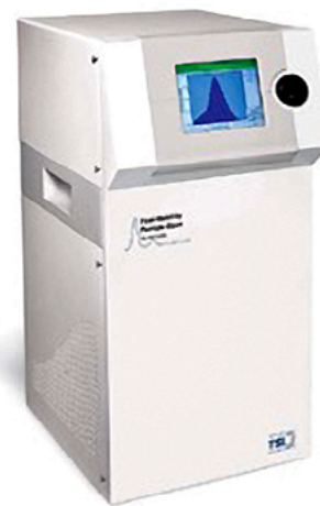
Figure 1. Equipment used in the Rieti campaign: Fast Mobility Particle Sizer, counting and size dimensional classification (electrical mobility diameter) 5.6-560 nm. Temporal resolution: 1 second
