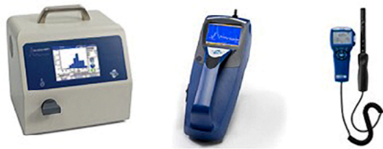
Figure 2. Mobile instruments used in the Venafro campaign: Nanoscan (left), DustTrak TM II aerosol monitor (middle) and Q-Trak TM Indoor Air Quality Monitors (right)
