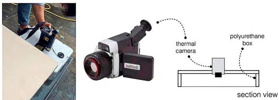
Figure 3. Surface temperature monitoring equipment and setting
