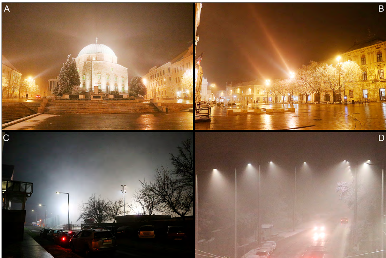
Figure 4. Negative and positive examples of lighting in Pécs (2019). The photos were taken in fog. Ornamental lighting and the reflectors of the stadium are largely directed above the horizon (A, B, C), while the new LED lamps fully below the horizon (D)
