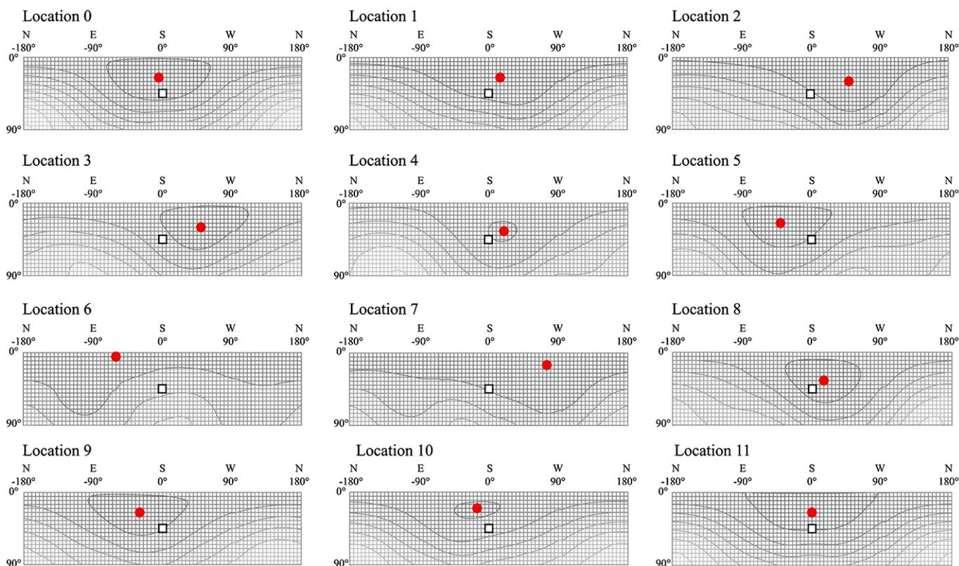
**Figure 8.** Distribution of insolation levels depending of the tilt and azimuth angles. Red circle shows maximal insolation obtained by approach and black square shows the values recommended by general rule
