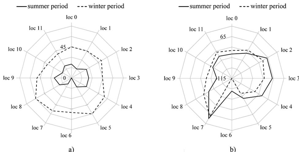
**Figure 10.** Comparison of the optimal: a) tilt angles; b) azimuth angles for summer and winter period
