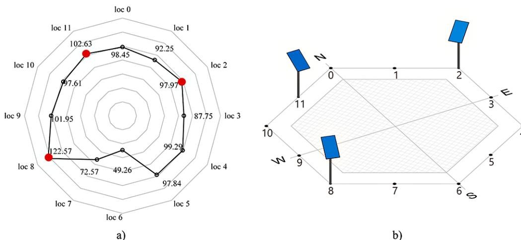
**Figure 11.** a) Maximal panel insolation for all locations. Selected combination is marked with red circles. b) Solar panel positions with maximal insolation level for whole year period at locations no. 2, 8 and 11
