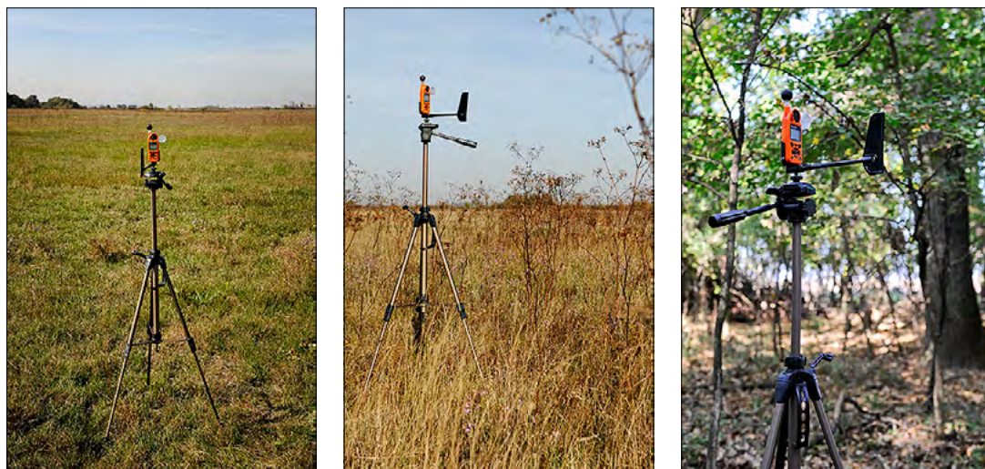
Figure 4. Instrumental set-up of the meteorological stations in: saline steppe, forest-steppe and forest (from left to right)
