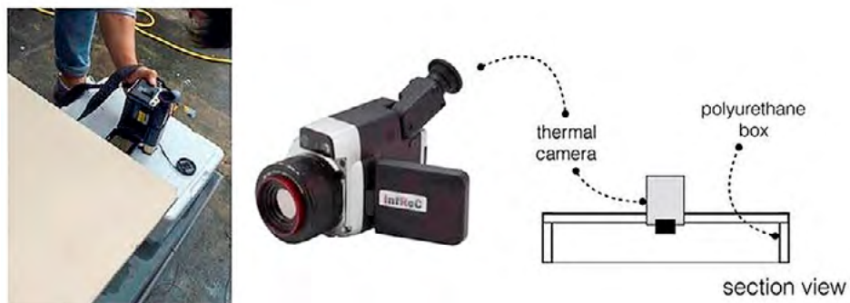
Figure 3. Surface temperature monitoring equipment and setting
