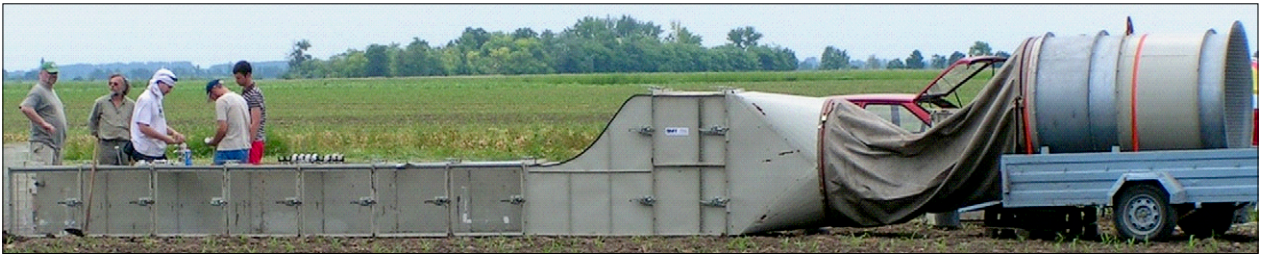
Figure 4. The portable wind tunnel
