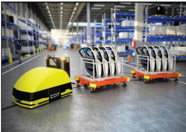
Figure 5: AGV system – towing version
