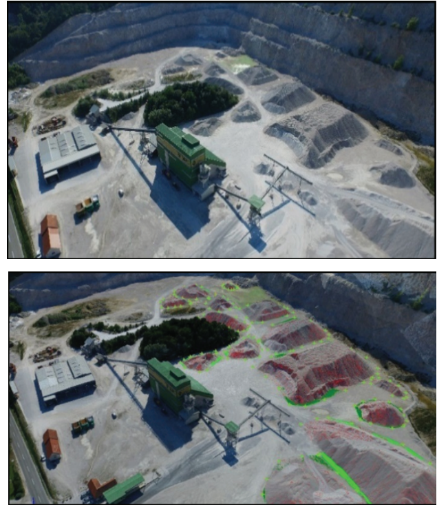
Figure 12: Realistic photograph of quarry (upper); 3D model generated from aerial photos using the UAV for measuring stocks (lower)
