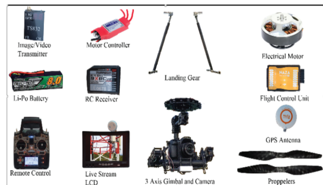
Figure 2: Major components of the developed multicopter (components are not in scale)
