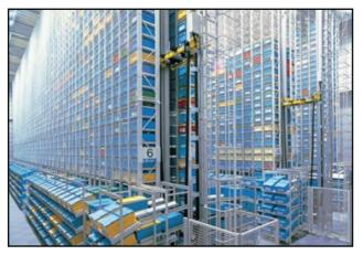
Figure 9: Automated Storage & Retrieval Systems (ASRS)
