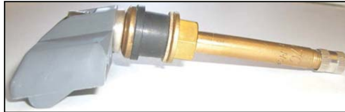
Figure 5: Sensor installed on valve stem
