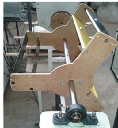
d) Tandem three bladed Darrieus turbine
