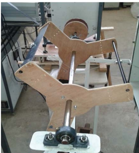
b) Three bladed Darrieus turbine
