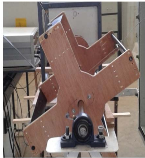
c) Four bladed Darrieus turbine
