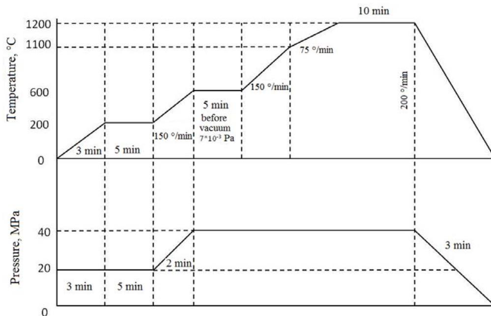
Figure 1: Consolidation of powders by the method of spark plasma sintering (scheme)
