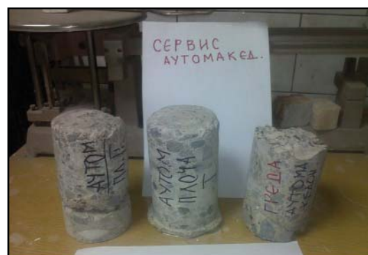
Figure 2. Three sample cylinders taken from the slab and the beams
