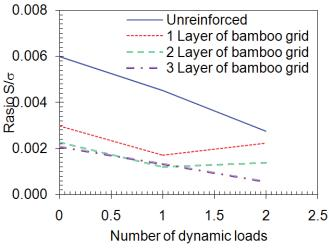
Figure 10: The relationship between ratio S/o and number of dynamic loads
