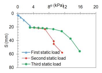
Figure 4: The relationship between S vs σ for unreinforced peat under static load
