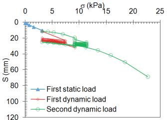
Figure 7: The relationship between S vs σ for reinforced peat under dynamic load
