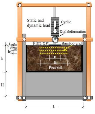
Figure 1: Model dimensions and bamboo grid configuration
