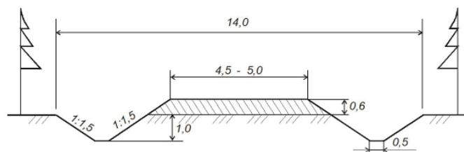
Figure 1: Cross-section structure of an earth fill erected by an excavator from side ditches, m
