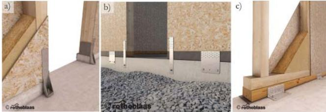
Figure 3: Examples of timber-framed walls anchoring to the concrete slab with a) angle brackets for tensile loads, b) straps for tensile loads and plates for shear loads c) angle brackets for shear loads (©rothoblaas)
