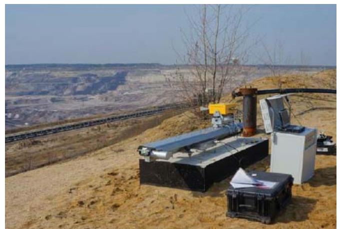
Figure 4: Radar IBIS L during measurement in open pit mine (photo A. Szafarczyk)
