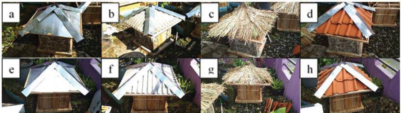
Figure 2: Roof variation of the building models, (a) Building with exposed stone wall and zinc roof; (b) Building with exposed stone wall and asbestos roof; (c) Building with exposed stone wall and thatch roof, (d) Building with exposed stone wall and roof tile; (e) Building with wood wall and zinc roof; (f) Building with wood wall and asbestos roof; (g) Building with wood wall and thatch roof; (h) Building with wood wall and roof tile.
