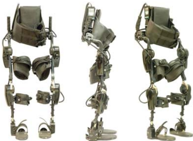
Figure 2: General view of Remotion exoskeleton
