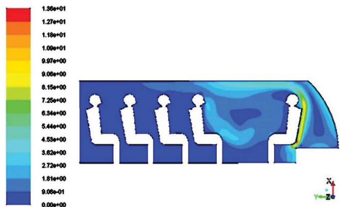
Figure 5: Distribution of air speed vector values in the passenger compartment of the wheeled vehicle without taking into account breathing of passengers
