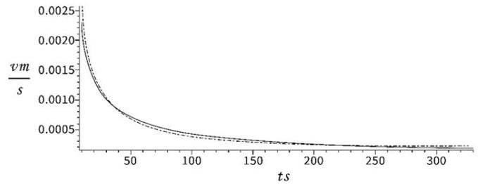
Figure 8: Impregnation rate for spruce samples ( $n = 900 \text{ rpm}$ ,  $\Delta = 0.2 \text{ m}$ )
