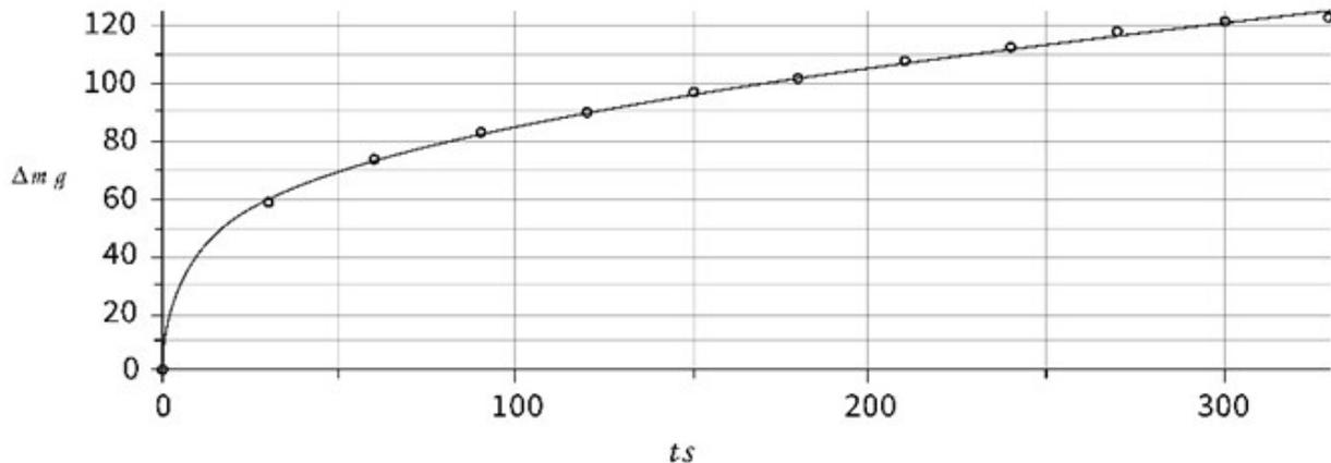
Figure 7: Change in the mass of spruce samples during impregnation ( $n = 900 \text{ rpm}$ ,  $\Delta = 0.2 \text{ m}$ )
