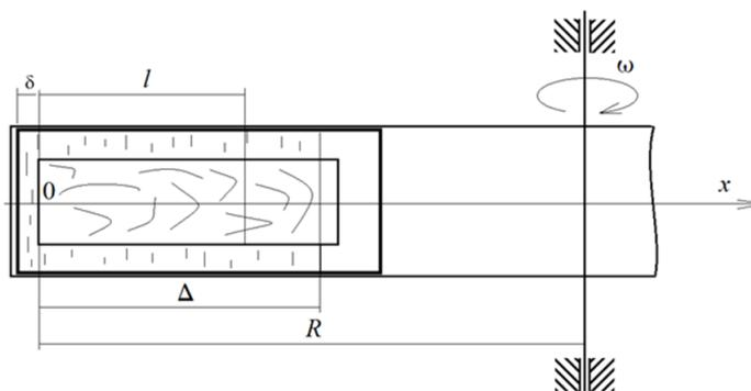
Figure 1: Scheme of oncoming-impregnation of the sample in the centrifugal force field
