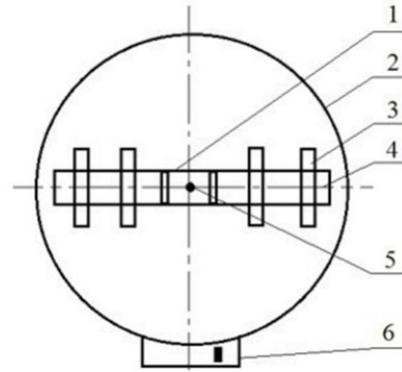
Figure 2. Scheme of the experimental plant: 1 – carousel; 2 – body; 3 – fastening half-rings; 4 – glass; 5 – axis of rotation; 6 – control panel
