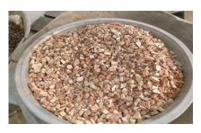
Figure 3: crushed ceramic aggregate
