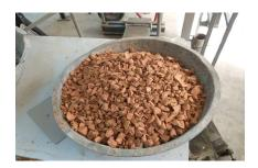
Figure 2: Clay brick aggregate
