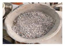
Figure 1: Recycled concrete aggregate
