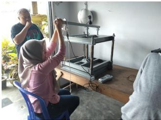
Figure 1: Pressing machine to mold the cassava dough
