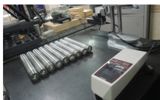
Figure 2: The setting of surface roughness measurement
