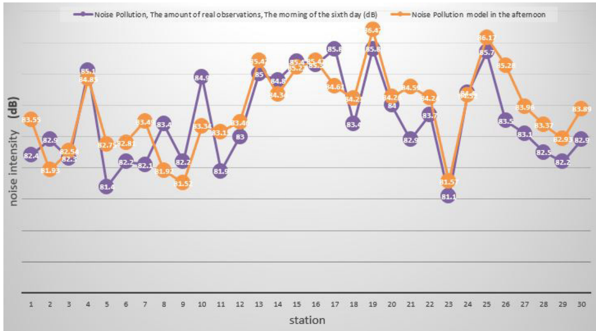
Figure 16: Comparison of noise intensity in the actual observations of the sixth day and the noise intensity model in the afternoon
