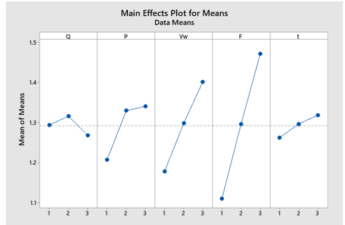
Figure 10: Main effects plot for means of R_q
