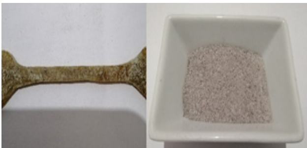
Figure 12: Mixture and tensile test specimen of PVC and cow horns
