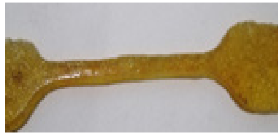
Figure 14: PVC & coconut tensile test specimen
