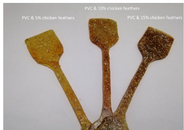
Figure 16: PVC & chicken feathers tensile test specimen
