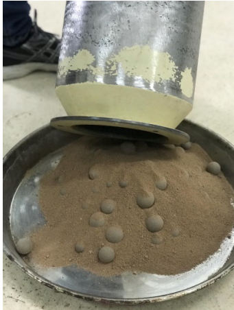
Figure 4: Feldspar passed from sieve #200 (0.075mm) and crushed by ball mill (used as a partial replacement material for cement)
