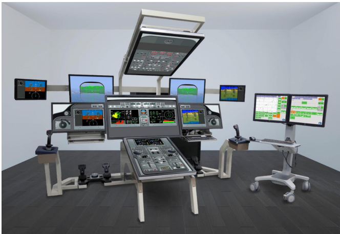
Figure 3: The Aircraft Cockpit Universal Prototyping Bench of GosNIIAS
