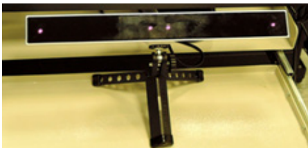
Figure 4: The eye tracker used for recording video oculography data
