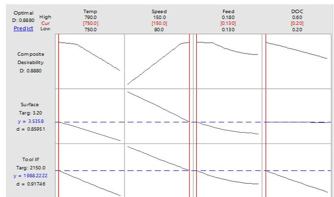
Figure 5: Response surface plots for TL and SR of AISI1040 F-B DPS
