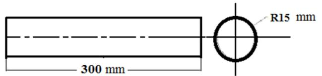
Figure 1: Test specimen details for machinability test
