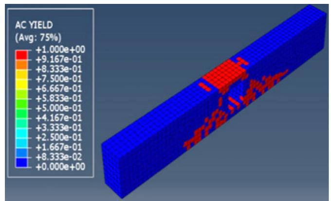
Figure 23: Yielding criteria on the RCB-CFRP-2L-W60
