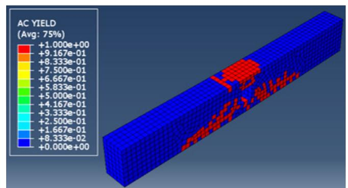
Figure 18: Yielding criteria on the RCB-W40
