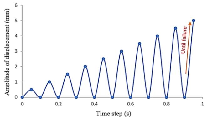
Figure 8: Amplitude of cyclic loading in different time steps of simulation
