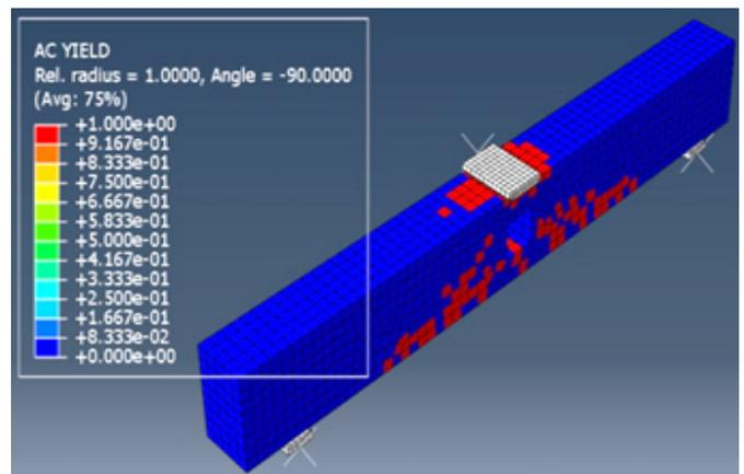
Figure 22: Yielding criteria on the RCB-CFRP-2L-W40
