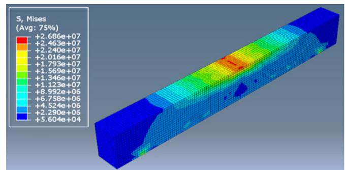
Figure 27: The maximum von Mises stress distribution on the RCB-CFRP-U after the 8th cycle
