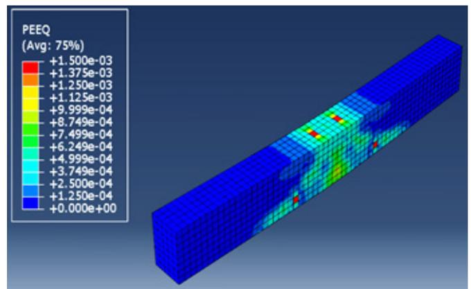
Figure 12: The equivalent plastic strain distribution on the reinforced concrete beam after the fifth cycle
