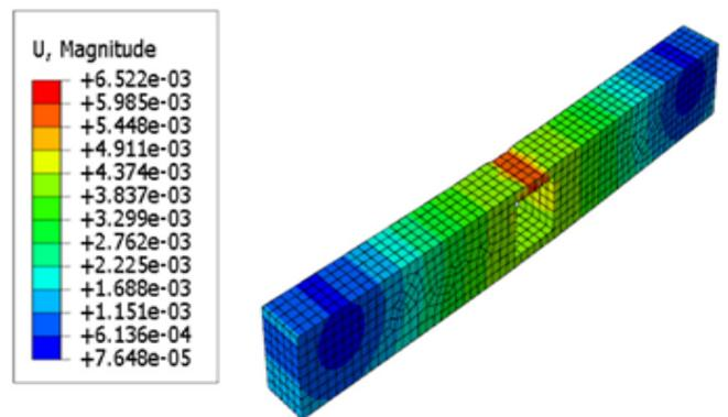
Figure 17: Localization of deformation on the top of the web opening part and failure of the RCB-W75 sample
