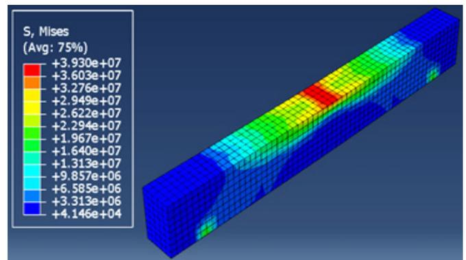
Figure 11: The maximum von Mises stress distribution on the reinforced concrete beam after the fifth cycle
