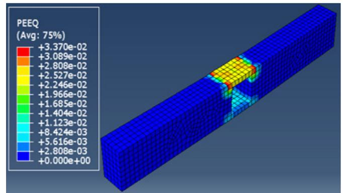
Figure 16: The equivalent plastic strain distribution on the RCB-W75 after the fourth cycle
