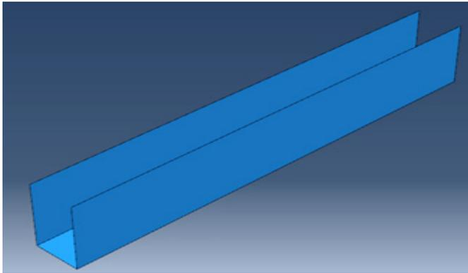
4-a: U shape wrapped CFRP
