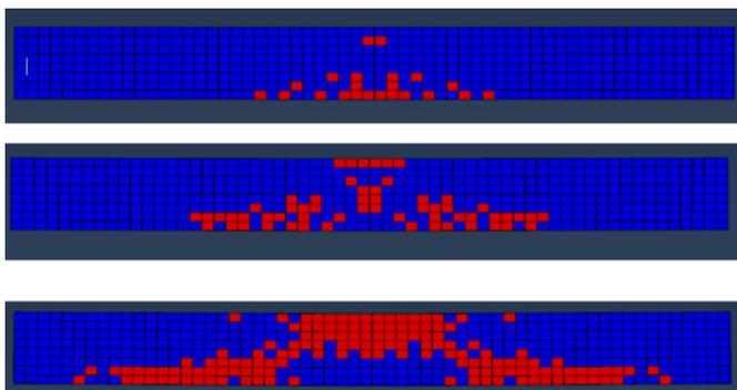
Figure 10: Yielding criteria stages on the RCB during the cyclic loading
