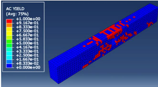
Figure 29: Yielding criteria of the RCB-CFRP-U-W40
