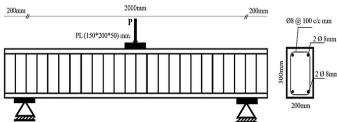
Figure 1: Details of RC beam includes bars and stirrups
