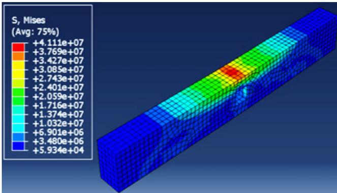
Figure 14: The maximum von Mises stress distribution on the RCB-W40 after the sixth cycle
