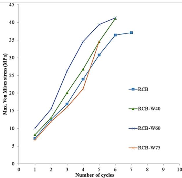
Figure 9: Maximum Von Mises stress of the RC beams with and without web opening at different cycles
