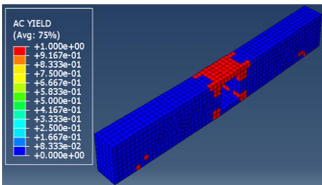
Figure 20: Yielding criteria on the RCB-W75
