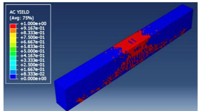
Figure 28: Yielding criteria of the RCB-CFRP-U under the flexural loading
