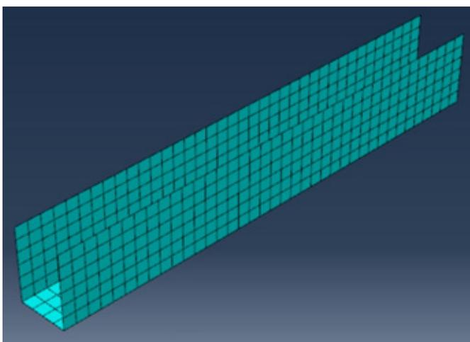
6-a: U shape wrapped CFRP
