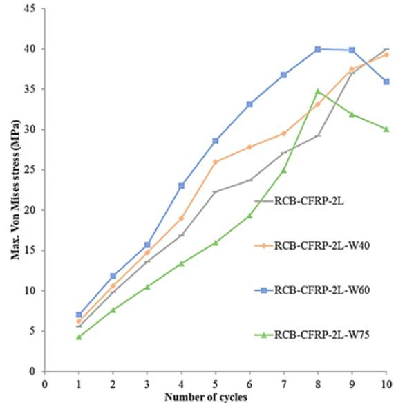
Figure 21: Maximum Von Mises stress of the RCB-CFRP-2L with and without web opening at different cycles
