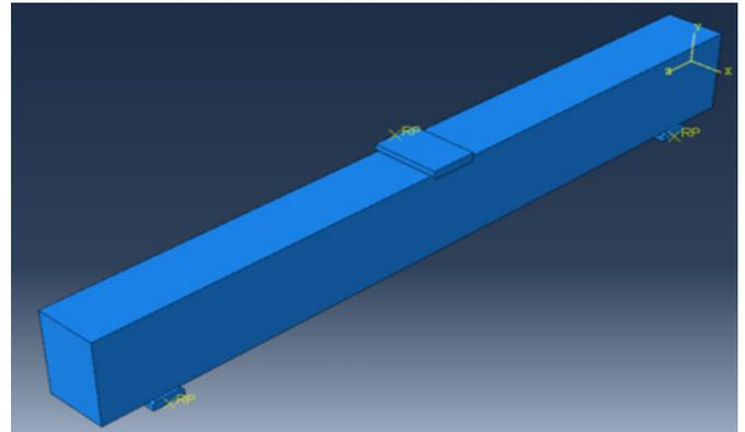
Figure 2: Assembly of the three-point bending system simulated in this study
