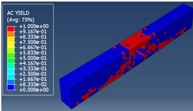
Figure 19: Yielding criteria on the RCB-W60
