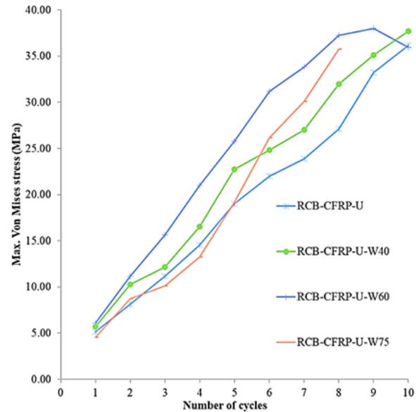
Figure 26: Maximum Von Mises stress of the RCB-CFRP-U with and without web opening at different cycles
