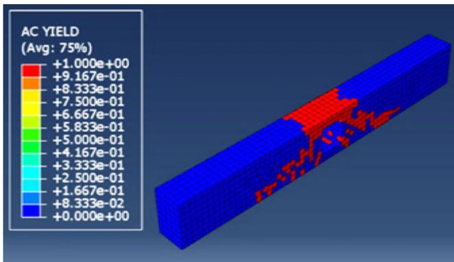
Figure 30: Yielding criteria on the RCB-CFRP-U-W60
