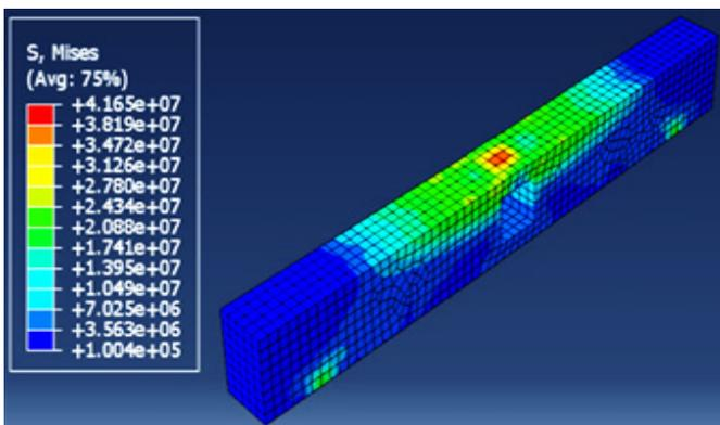
Figure 15: The maximum von Mises stress distribution on the RCB-W60 after the sixth cycle
