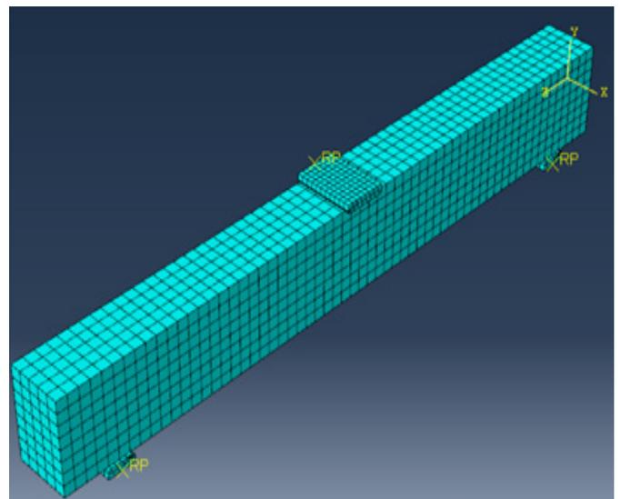
Figure 5: Meshed setup
