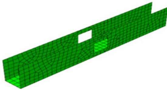
7-a: mesh of CFRP laminates with opening
