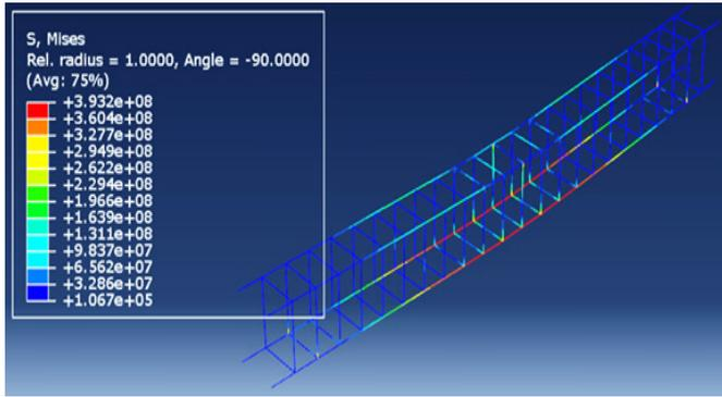
Figure 13: The maximum von Mises stress distribution on the reinforced concrete beam
