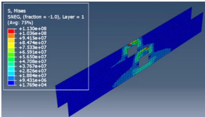
Figure 25: The maximum von Mises stress distribution on the CFRP laminates of RCB-CFRP-2L-W60
