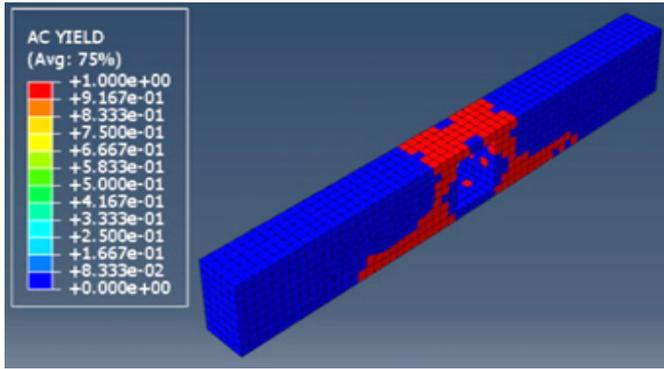
Figure 24: Yielding criteria on the RCB-CFRP-2L-W75
