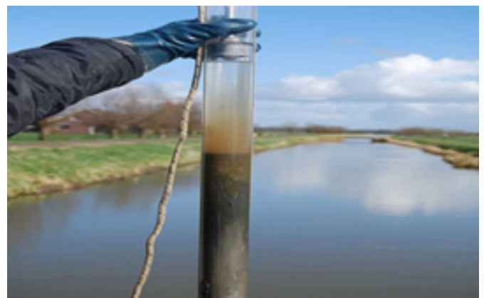
Figure 3: View at the irrigation canal and Beeker sampler filled with sediments
