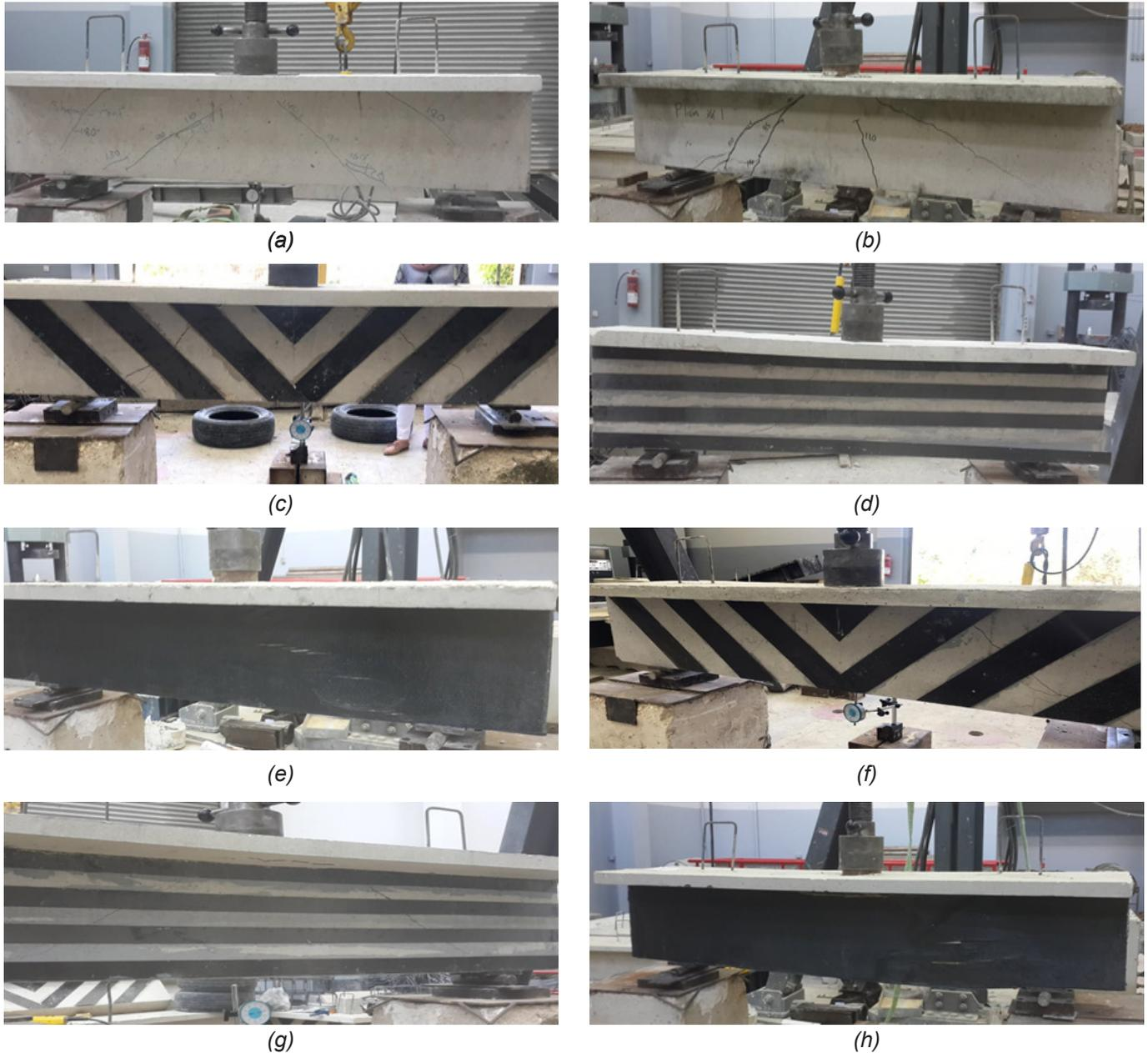
Figure 8: Crack patterns for beams: (a) CB; (b) PB1; (c) SB1; (d) SB2; (e) SB3; (f) RB1; (g) RB2; (h) RB3
