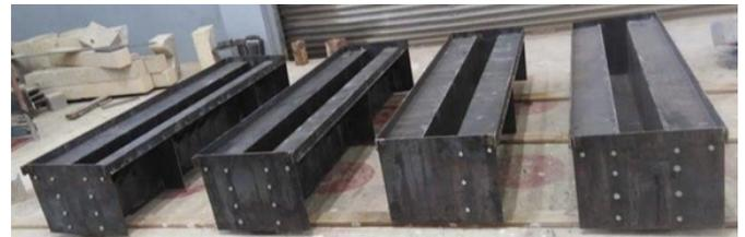
Figure 4: Formwork used for all specimens
