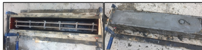
Figure 2: The Photos of the Moulds with the concrete cast within
