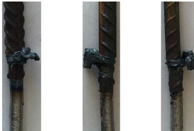
Fig. 5. \varnothing 10\text{ mm} sample welded in mode 1 ( t_r=25\text{s} , n=1600\text{ rpm} ).
