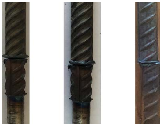
Fig. 6. \varnothing 14\text{mm} sample welded in mode 2 ( t_r=30\text{s} , n=2000\text{ rpm} ).
