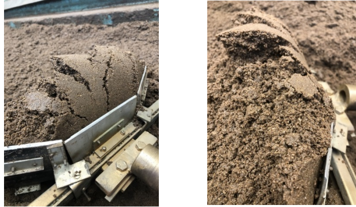
Fig. 7. Digging the soil with a blade with variable geometry with an angle of \theta=30^\circ .
