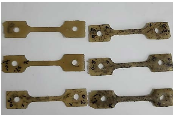
Fig. 4 Creep samples in different Weight fraction
