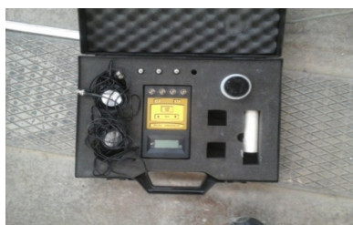
(c) Ultrasonic pulse velocity apparatus used
