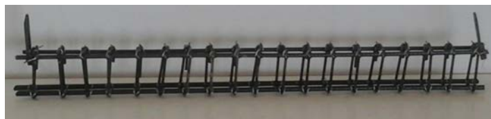
Fig. 2. Beam reinforcement of the specimen
