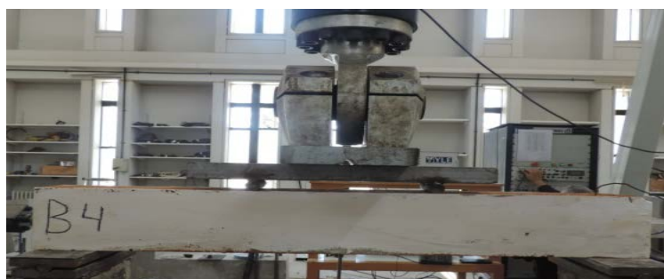
Fig. 6. Four-point flexural test setup
