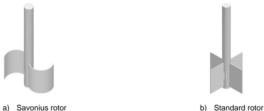
Figure 3. Savonius rotor
