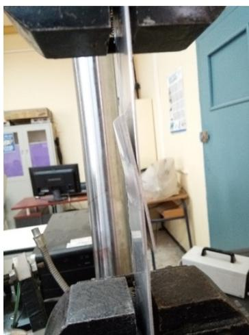
Fig.7. Shear specimen during the tensile test
