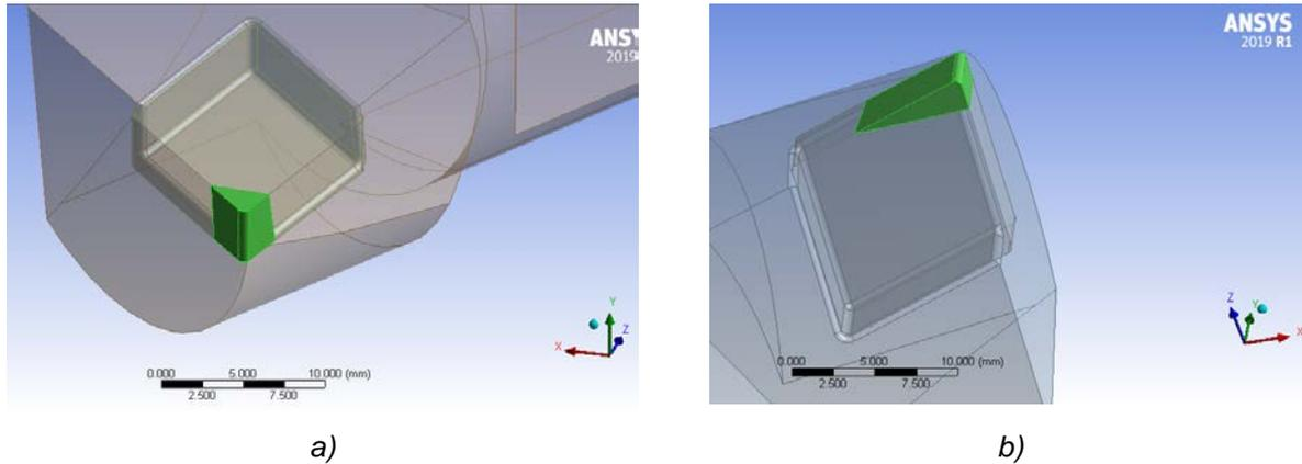
a) - 60° for boring a hole with a diameter of 295 mm; b) - 80° for boring a hole with a diameter 325mm
