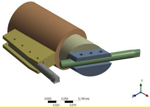
Fig. 14. Three-dimensional model of a boring bar with optimal parameters
