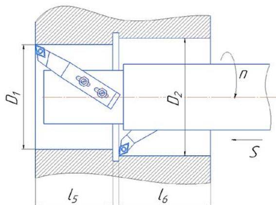
Fig. 2. drawing of the process of boring stepped holes
